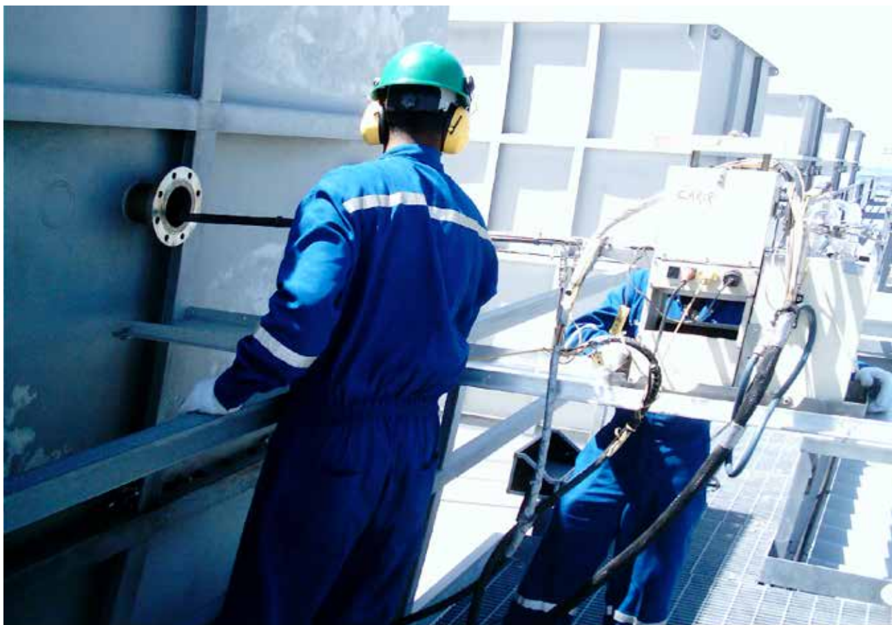
Stack Emission Monitoring of Turbine Compressors on the Facility
