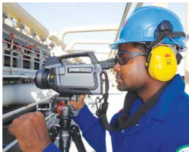
The FLIR GF 320 Optical Gas Thermal Imager is now part of our proactive approach to leak management and prevention
